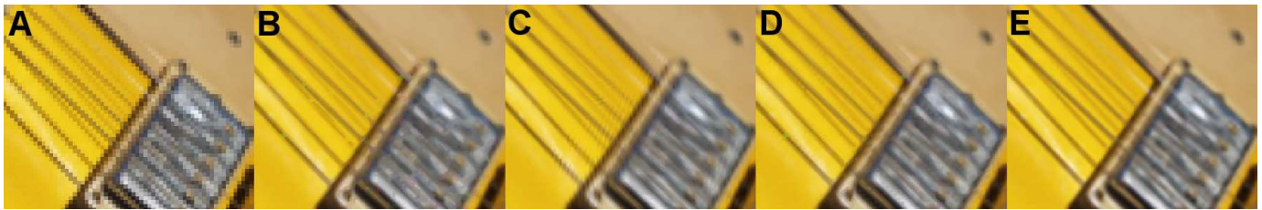
Fig. 5. Comparison of different "edge directed" interpolation methods. A: Image detail enlarged ( 4\times ) with pixel replication. B: the same detail enlarged by a 4\times factor with Chen's edge directed method. C: the same detail enlarged with NEDI method. D: the same enlargement obtained with our fast curvature based interpolation method (FCBI). E: the same enlargement obtained with our iterative curvature based iterative interpolation method (ICBI).
